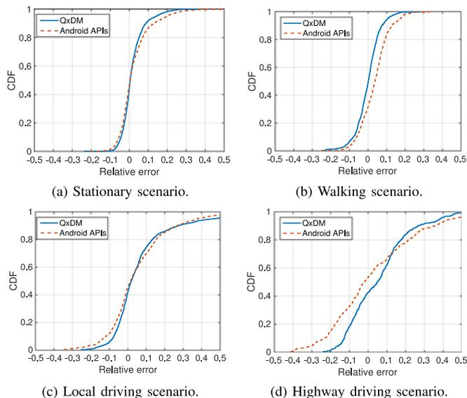
Fig. 15. Prediction errors when using data collected through Android APIs in comparison with the results when using data collected through QxDM.
