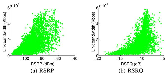
Fig. 2. Scatter plot of RSRP, RSRQ, and link bandwidth for the highway driving scenario.
