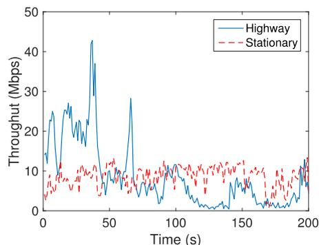
Fig. 1. Illustration of rapidly changing link bandwidth in LTE networks.
