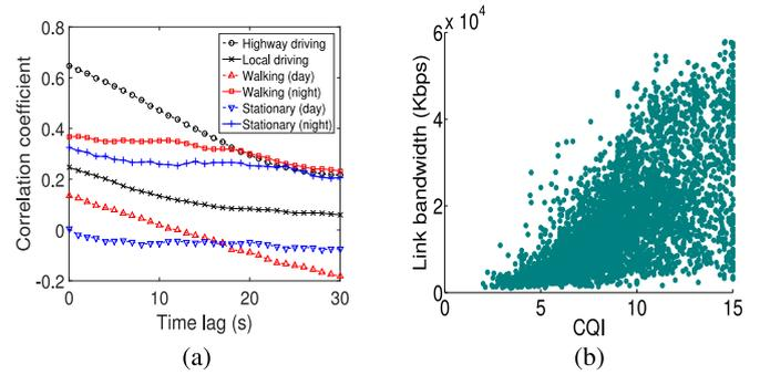
Fig. 5. (a) Correlation coefficient between CQI and link bandwidth for various scenarios. (b) Scatter plot of link bandwidth and CQI in the highway driving scenario.
