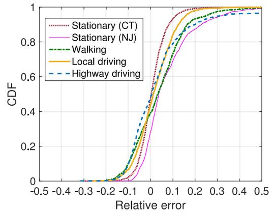
Fig. 10. Relative prediction error in various mobility scenarios (using Samsung Note 3 on AT&T network).
