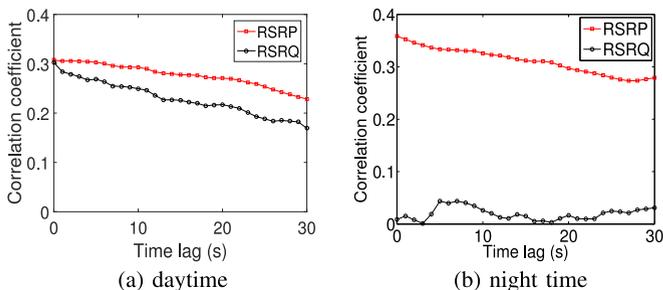
Fig. 4. Correlation coefficient between RSRP, RSRQ, and link bandwidth for the stationary scenario (data collected on campus).
