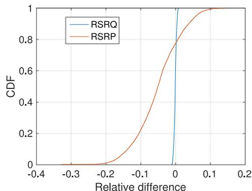
Fig. 14. Relative differences of the values collected using Android APIs and those collected using QxDM.
