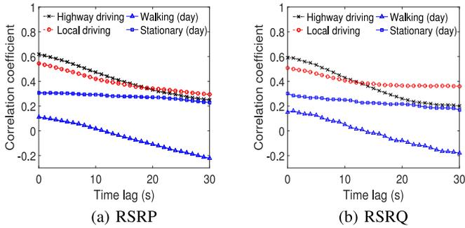
Fig. 3. Correlation coefficient between RSRP, RSRQ, and link bandwidth for various scenarios.
