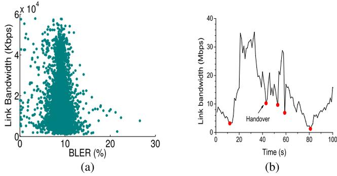
Fig. 6. (a) Scatter plot between link bandwidth and BLER (highway driving scenario). (b) Link bandwidth and handover events.
