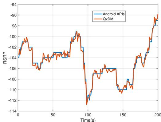
Fig. 13. Comparison of RSRP values collected using QxDM and Android APIs.
