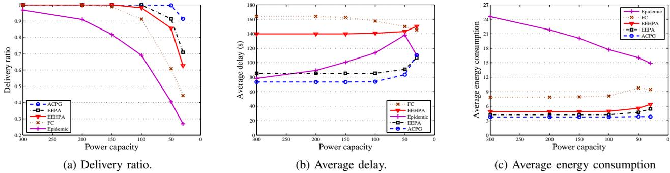
Fig. 4. Performance comparison of various routing schemes in UWSN with regular currents.
