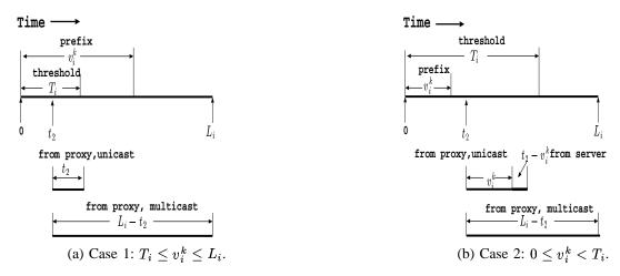
Fig. 6. Delivery to proxy k, which initiates the transmission of suffix from the server using multicast in MMPatch.
