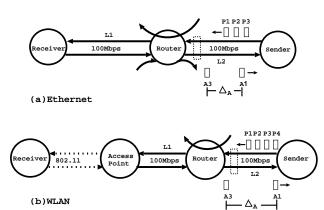
Figure 2: Settings for the analysis: (a) Ethernet, (b) WLAN (802.11b or 802.11g). The dashed rectangle between the sender and the router represents the monitoring point. The pair of ACKs,  $A_1$  and  $A_3$ , forms an ACK-pair.
