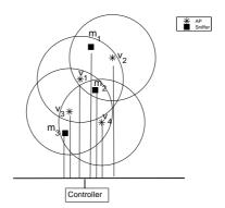
Fig. 1. Problem setting: a central controller controls the channels of the APs and determines the channel assignment for the sniffers.
